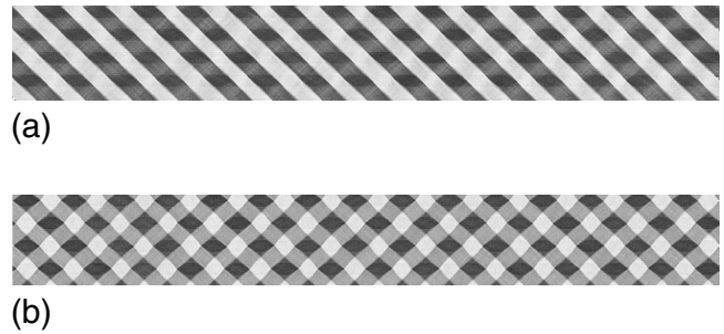
FIG. 5. Microstructures of rectangle-rectangle nanocomposites with 100-nm-thick layers at 258 K and (a) x_a=0.23 and (b) x_a=0.24 . Gray: austenite; black and white: (rectangular) martensite.
